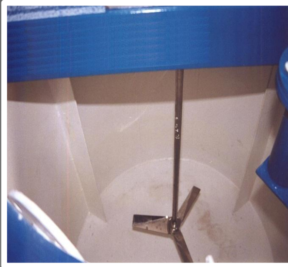
Baffled, mechanically agitated mixing tank (no air agitation)
