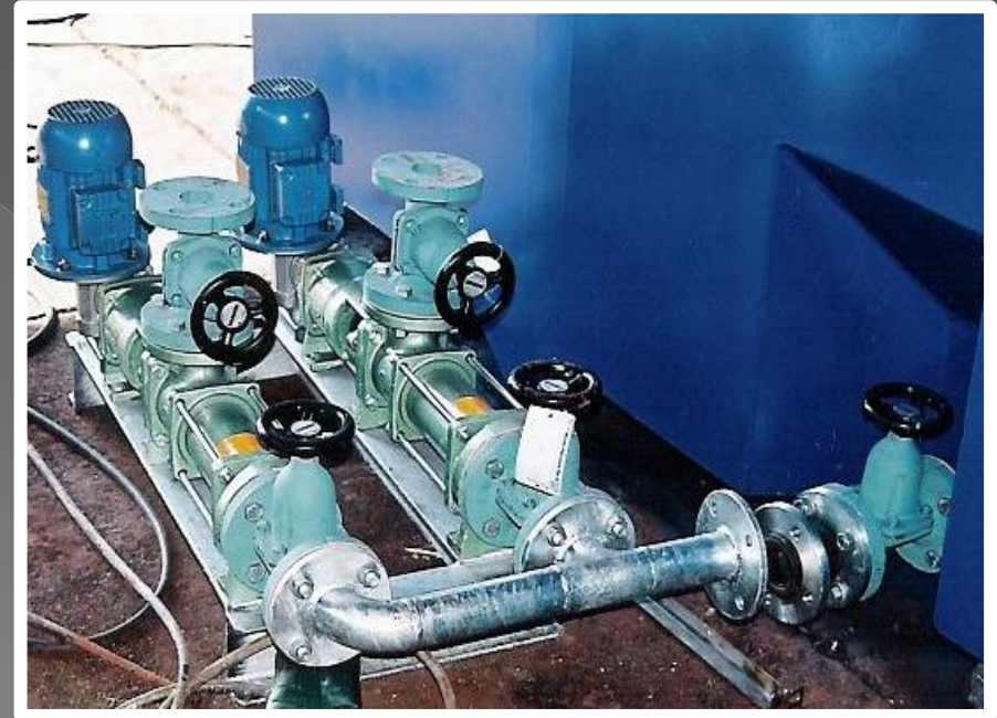
Dosing pump-mounting base, all valves, flanges and internal connecting piping
